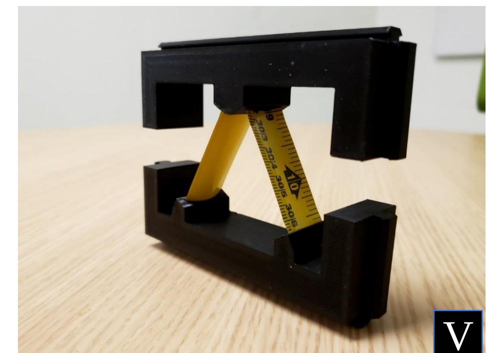
(V) A single PXCm cell with a tape spring ligament as a constituent.
